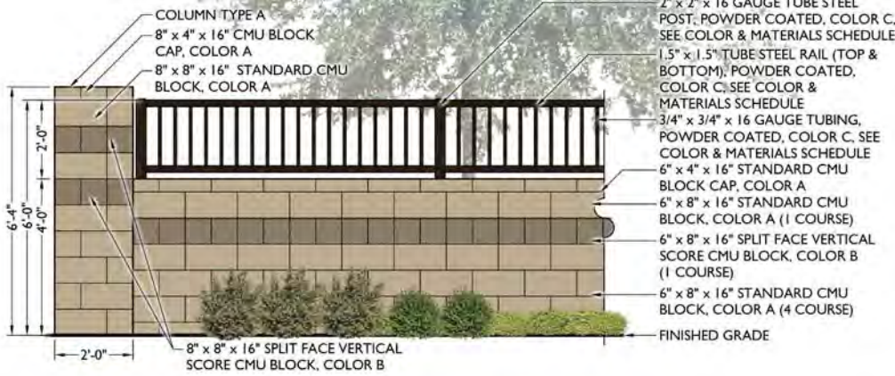
4 PARTIAL VIEW WALL Scale: 1/2" = 1'-0"
