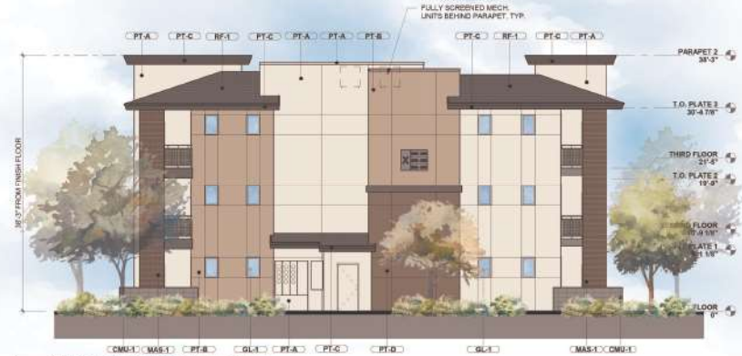
3 BUILDING 1 RIGHT ELEVATION 1/8" = 1'-0"
