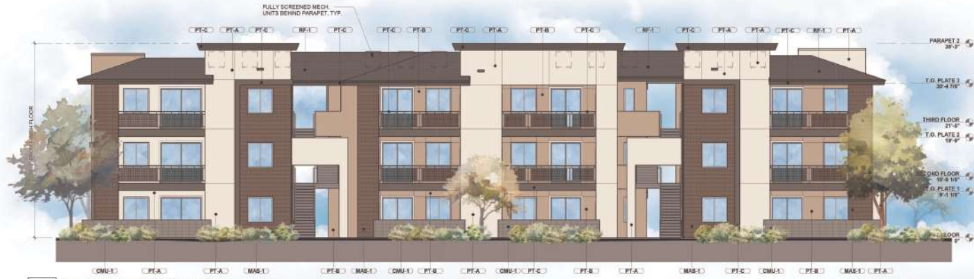
1 BUILDING 1 FRONT ELEVATION 1/8" = 1'-0"
