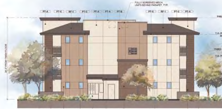
3 BUILDING 1 RIGHT ELEVATION 18' x 1'-0"
