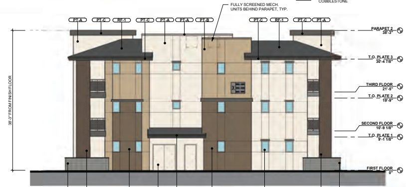
3 BUILDING TYPE 1 RIGHT ELEVATION 18' = 1'-0"
